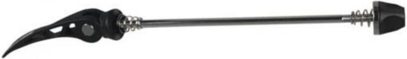
Remove the nut and one spring from the quick release skewer. Now from the disc side insert the skewer and from the other side attach one spring followed by the nut. The springs are there just simply to help you to align the skewer so that it sits easily in the dropouts.
