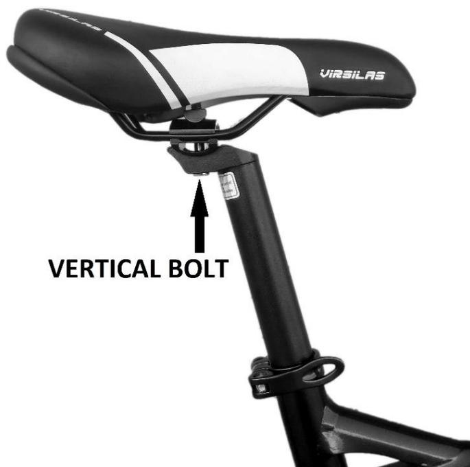
Loosen the large, vertical bolt on the seat clamp with a hex wrench. This loosens a clamp that secures the seat rails. Loosen it until you can spin the top of the clamp. Spin it 90 degrees and you'll be able to insert the seat. Now insert the rails of your seat into the grooves on the bottom of the seat clamp. Adjust the top of the clamp onto the rails and tighten the bolt slightly so that the hardware is in place.
